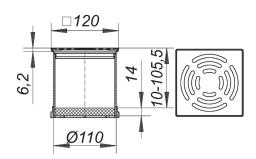
used with floor drain bodies types 40, 42 and 46, with balcony drain bodies types 83 and 84, drainage elements for attic drains as well as type 85 raising piece, spigot ABS, extendable with DN 100 plastic pipe, frame 304 stainless steel,  $120 \times 120 \text{ mm}$ , grate 304 stainless steel, load class K 3 (300 kg)
